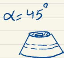
$$k_m = \frac{\pi d E}{\ln \left[ \frac{(2t + D - d)(D + d)}{(2t + D + d)(D - d)} \right]}$$
