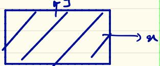
$$\begin{Bmatrix} \alpha_x \\ \alpha_y \\ \alpha_{xy} \end{Bmatrix} = [T(\theta)]^{-1} \begin{Bmatrix} \alpha_1 \\ \alpha_2 \\ \alpha_3 \end{Bmatrix}$$
