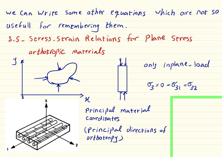
The strain stress relation for orthotropic materials
