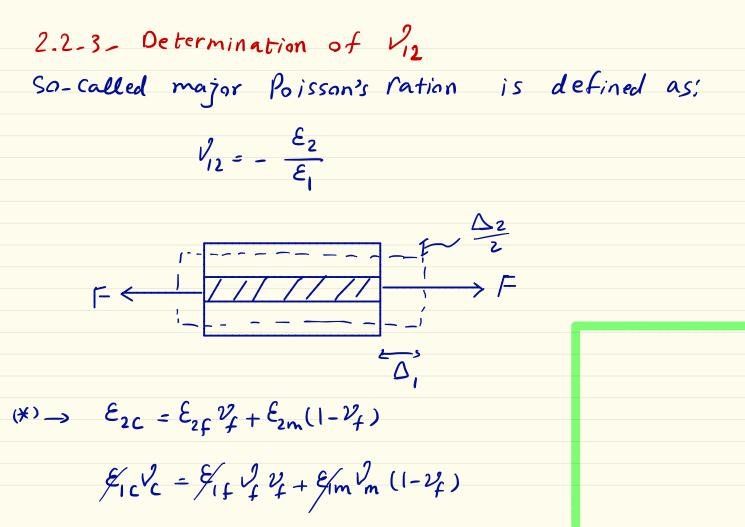
$$v_{c} = v_{f}v_{f} + v_{m}(1 - v_{f})$$
