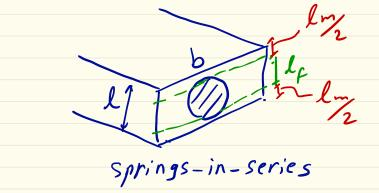
$F_{c} = F_{m} = F_{f} \longrightarrow \tilde{c} = \tilde{c}_{m} = \tilde{c}_{f}$ Dc=Dm+Df -> Ec. l=Ef.lf+Emlm  $(\bigstar) \ \mathcal{E}_{c} = \mathcal{E}_{f} \ \mathcal{V}_{f} + \mathcal{E}_{m} (1 - \mathcal{V}_{f})$  $\frac{\overline{\mathcal{D}_{2C}}}{E_{2C}} = \frac{\overline{\mathcal{D}_{2f}}}{E_{f}} \frac{\mathcal{D}_{f}}{\mathcal{D}_{f}} \frac{\mathcal{D}_{2m}}{E_{m}} (1 - \mathcal{D}_{f})$
