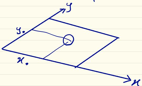
$$\frac{\partial^4 w}{\partial x^4} + 2 \frac{\partial^4 w}{\partial x^2 \partial y^2} + \frac{\partial^4 w}{\partial y^4} = \frac{P(x, y, t)}{D} \quad (h)$$
