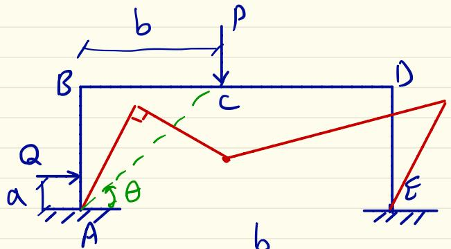
$$Qa\omega + P(\text{AC} \cdot \sin \theta) \omega = \underbrace{\omega M_p}_{(A)} + \underbrace{2\omega M_p}_{(C)} + \underbrace{2\omega M_p}_{(D)} + \underbrace{\omega M_p}_{(E)}$$
