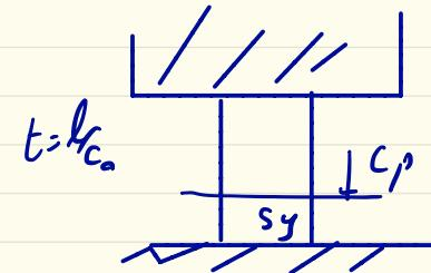
$$\begin{aligned}\sigma_R &= f C_p \Delta v = f C_p (0 - (-C_0 \epsilon_j)) \\ \rightarrow \sigma &= S_y + \sigma_R = S_y + f C_p C_0 \epsilon_j = S_y \left(1 + C_p C_0 \frac{f}{E}\right) \\ \rightarrow \sigma &= S_y \left(1 + \frac{C_p}{C_0}\right)\end{aligned}\quad (5-8)$$
