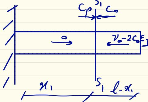
$$T_1 = \frac{x_1}{C_p} = \frac{l + (l - x_1)}{C_0}$$
