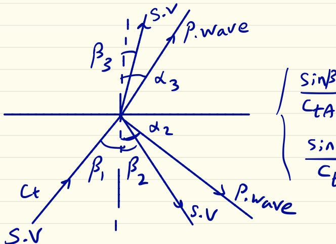
$$\left\{ \begin{array}{l} \frac{\sin \beta_1}{c_{tA}} = \frac{\sin \beta_2}{c_{tA}} = \frac{\sin \alpha_2}{c_{dA}} \\ \frac{\sin \beta_1}{c_{tA}} = \frac{\sin \beta_3}{c_{tB}} = \frac{\sin \alpha_3}{c_{dA}} \end{array} \right.$$
