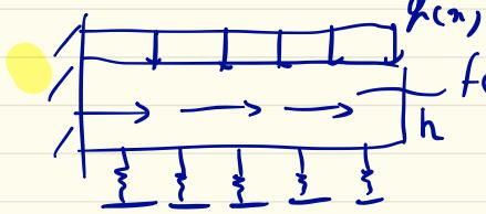
$$\delta W_E = - \left[ \int_0^L (f(n) \delta U_0 + q(x) \delta W(x, \frac{h}{2})) dx \right. \\ \left. + \int_0^L F_s \delta W(x, \frac{h}{2}) dx \right] \quad (9.4-4)$$
