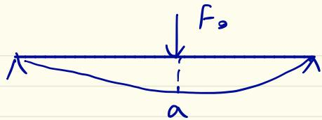
$$u = u_0 + z\phi \xrightarrow{\text{متارن}} \phi_n\left(\frac{a}{2}\right) = 0 \Rightarrow C_1 = -\frac{F_0 b a^2}{16 E_x^b I_y}$$
