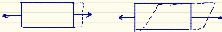
$$\begin{Bmatrix} \varepsilon_1 \\ \varepsilon_2 \\ \vdots \\ \delta_{12} \end{Bmatrix} = \begin{bmatrix} s_{11} & s_{12} & s_{13} & 0 & 0 & s_{16} \\ s_{12} & s_{22} & s_{23} & 0 & 0 & s_{26} \\ s_{13} & s_{23} & s_{33} & - & - & s_{36} \\ 0 & 0 & 0 & - & - & s_{46} \\ s_{16} & s_{26} & s_{36} & - & - & s_{66} \end{bmatrix} \begin{Bmatrix} \sigma_1 \\ \sigma_2 \\ \vdots \\ \gamma_{12} \end{Bmatrix}$$
