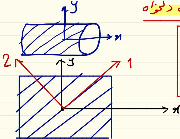
$$\begin{Bmatrix} \sigma_x \\ \sigma_y \\ \gamma_{xy} \end{Bmatrix} = [\bar{Q}] \begin{Bmatrix} \varepsilon_x \\ \varepsilon_y \\ \gamma_{xy} \end{Bmatrix}$$
