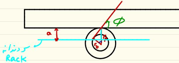
$$a = r_p - r_b \cos \phi = r_p - r_p \cos^2 \phi = r_p (1 - \cos^2 \phi)$$
