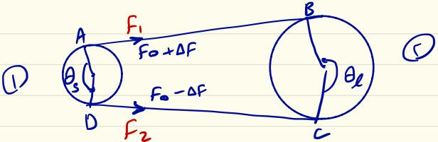
$$\left\{ \begin{array}{l} F_{max1} = F_1 + F_{C1} + F_{b1} \\ F_{max2} = F_2 + F_{C2} + F_{b2} \end{array} \right.$$
